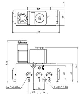
\* Minimum height with plug connector rotated through 90 degrees.
