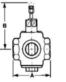
Fig. 200L, 200T - Sizes <sup>1</sup>/2" to 2" > 4" size has bolted cover
